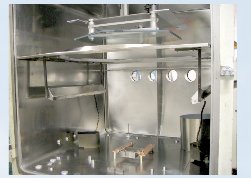
Interior of the aluminizing chamber.
